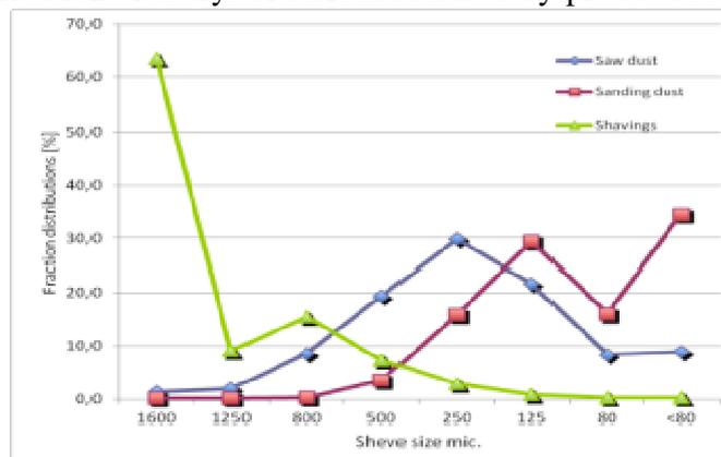
Figure 1: wood-based by-products sieve analysis
