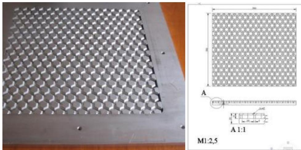
Figure 2. The hexagonal press tool and the aluminium frames
