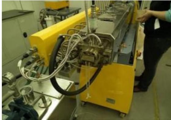
*Figure 5: The extruder used for PP and wood compounding*
