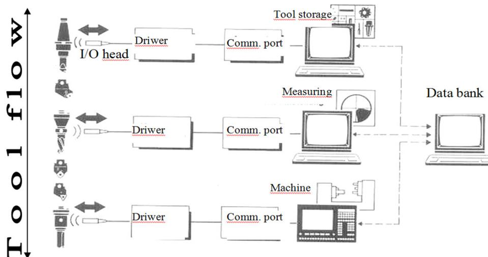
Figure 3. Read-write system installed into the tool
