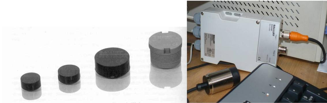
*Figure 1. EPROM media, Read/Write head and evaluation unit*
