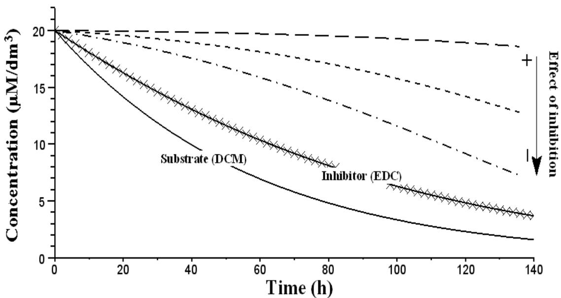
Figure 1. Effect of inhibition on the degradation of substrate (DCM), (Kinetic curves under inhibitor EDC with broken lines)
