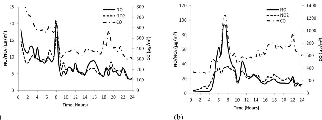
Figure 1. Concentration of CO, NO, NO<sub>2</sub>, represented as 30-minute averages, measured at busy street in Sopron (a) on 26 March 2011, (b) on 10 October 2011.
