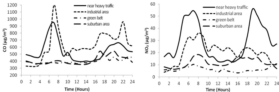
Figure 4. Typical day CO and NO<sub>2</sub> curves at selected locations in Sopron in October 2011
