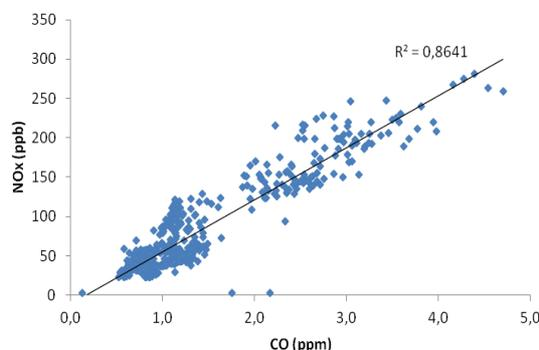
*Figure 6. Concentration of CO versus NO<sub>x</sub> for November 2011 measured in Székesfehérvár*
