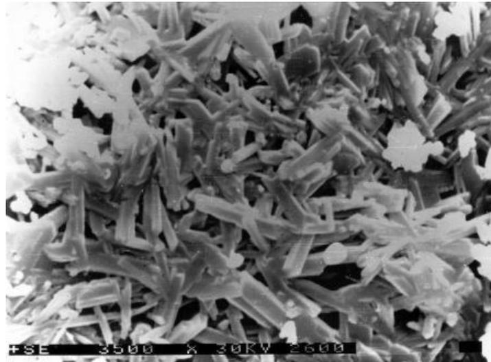
Figure 1. Lime sludge (Amplification: 3500 fold)
