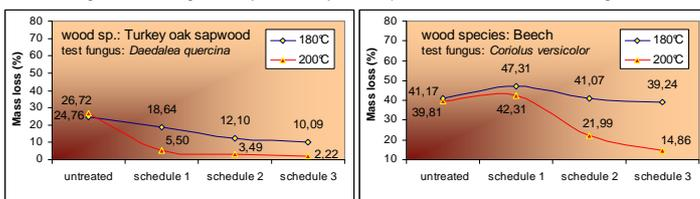
Figure 1. Average mass loss of Turkey oak sapwood and beech caused by wood destroying fungi (lines are for guiding the eyes)
