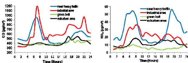
Figure 2. Typical day CO and NO<sub>2</sub> curves at selected locations in Sopron in October 2011
