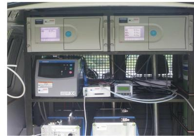
Figure 1. Mobile air testing equipment for immission analysis
