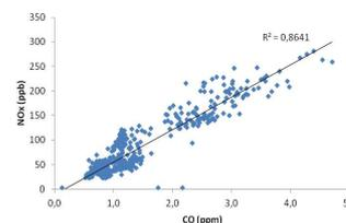
Figure 5. Concentration of CO versus NO<sub>x</sub> for November 2011 measured in Székesfehérvár
