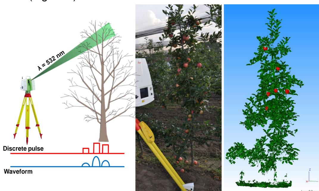
**Figure 1.** The principle of laser scanning with echoes and the model of a chosen tree in 3DReshaper software environment
