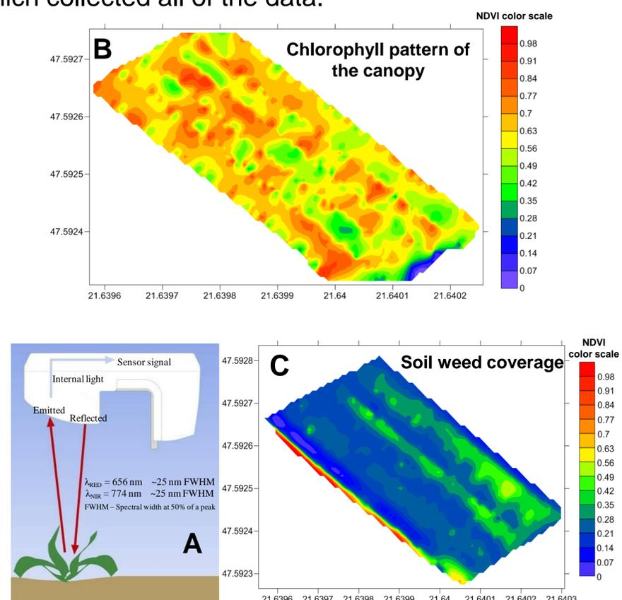
**Figure 2.** Working principle of GreenSeeker 505 (A), NDVI canopy map (B) and NDVI soil map (C) of the investigated apple orchard
