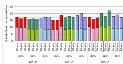
Fig. 2: The effect of treatment parameters on the Brinell-Möörth hardness
