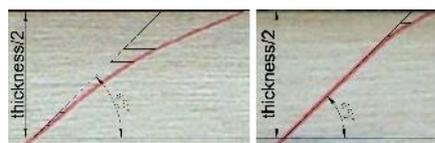
Fig. 7: The densification of different layers due to densification values of 40% (left) and 20% (right)
