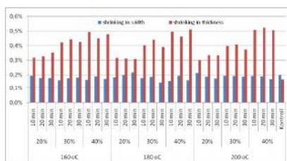
Fig. 5: The effect of treatment parameters on the shrinking coefficient in width and in thickness
