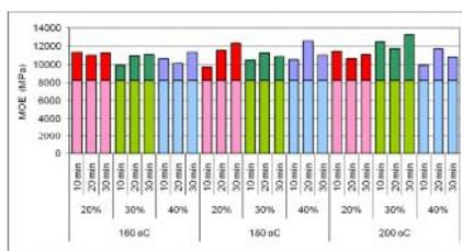
Fig. 4: The effect of treatment parameters on the MOE
