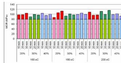
Fig. 3: The effect of treatment parameters on the MOR
